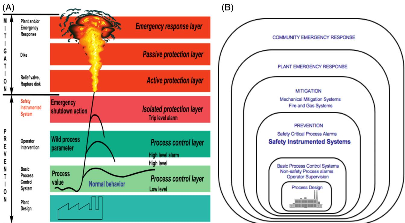
**FIGURE 2** Mitigation and prevention layers of protection determined in process hazard analysis (PHA) studies<sup>1</sup> [Color figure can be viewed at wileyonlinelibrary.com]
