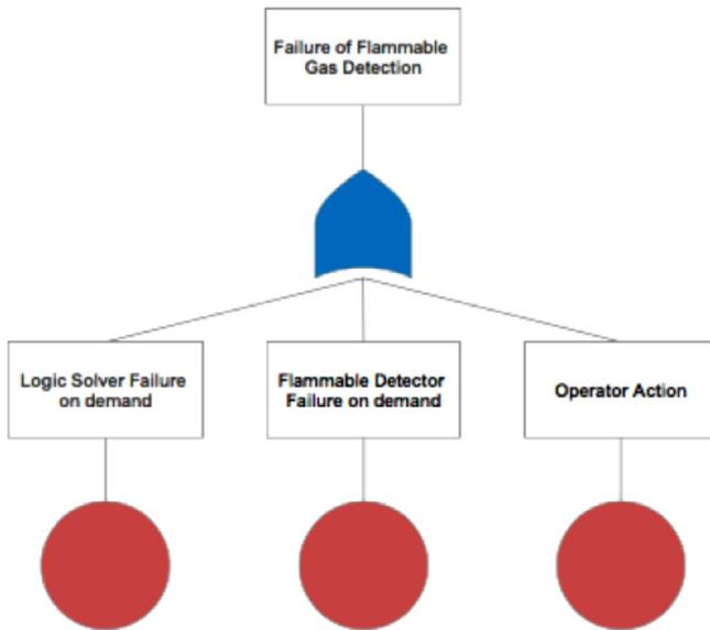
**FIGURE 5** Fault tree analysis for flammable gas detection [Color figure can be viewed at [wileyonlinelibrary.com](http://wileyonlinelibrary.com)]
