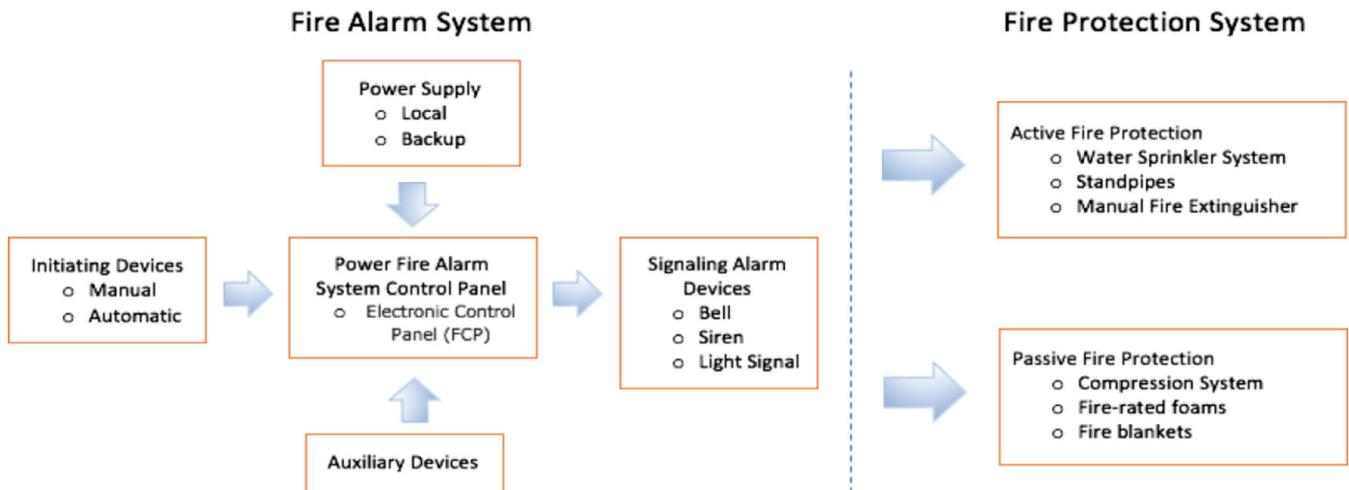
**FIGURE 1** Fire alarm system and fire protection system [Color figure can be viewed at wileyonlinelibrary.com]
