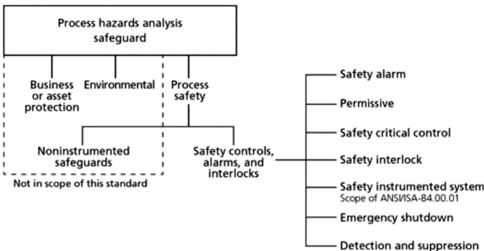
**FIGURE 3** Safety controls, alarms, and interlocks relationship to the process hazard analysis (PHA)<sup>2</sup>
