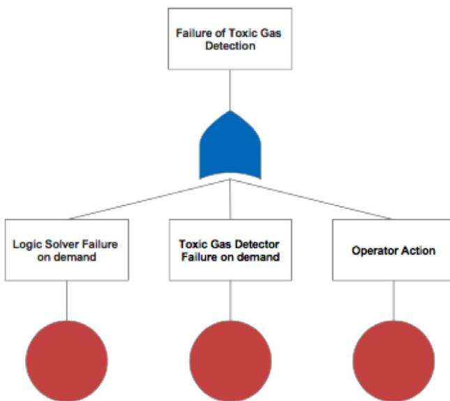
**FIGURE 6** Fault tree analysis for toxic gas detection [Color figure can be viewed at [wileyonlinelibrary.com](http://wileyonlinelibrary.com)]
