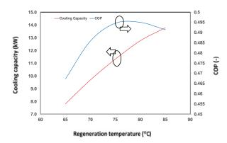
**Figure 5.** Effects of regeneration temperature on cooling capacity and COP
