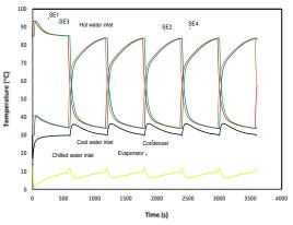
**Figure 3.** Temperature profiles for various components of silica gel-water cycle at rated conditions
