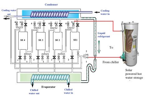
1: Hot water outlet; 2: Coolant inlet to the adsorber; 3: Hot water inler; 4: Coolant outlet from the adsorber
