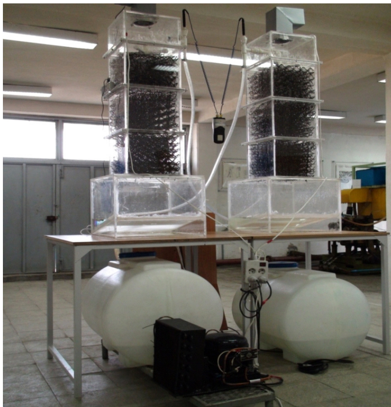
Figure 2. Main components of a packed bed liquid desiccant cooling system
