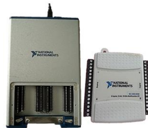
Fig. 2. NI-DAQ –X Series and NI-USB 6008 Signal Genration Unit for EEG Simulation.
