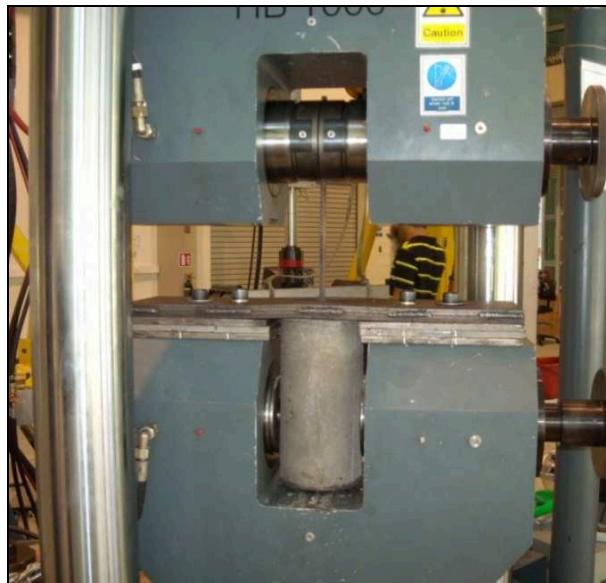
Fig.1 Pull out test setup
