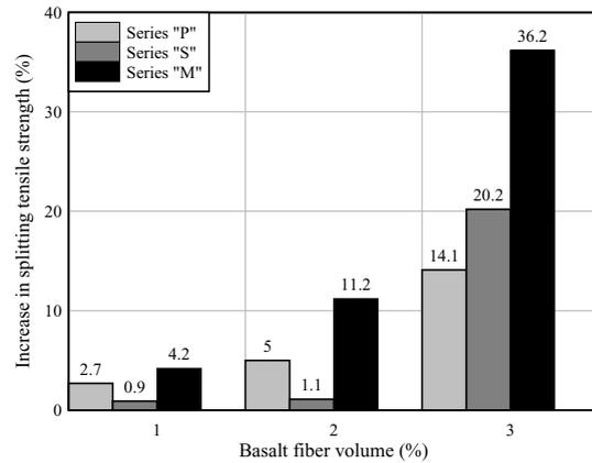
Fig. 8. Increase in splitting tensile strength with respect to control
