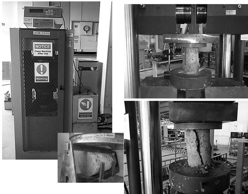
Fig. 4. 100×200 mm cylinder testing for (a) splitting tensile strength; (b) compressive strength.
