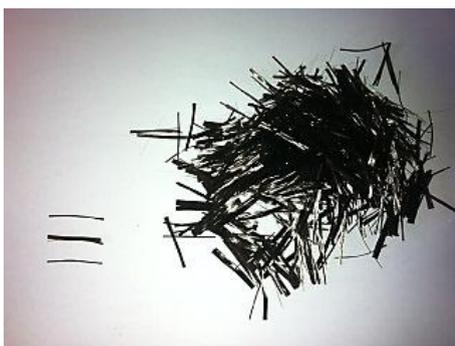
Fig. 2. Chopped Basalt fiber.
