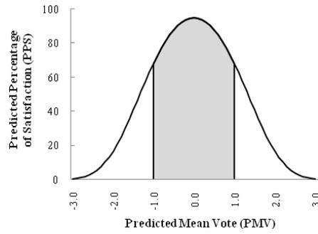
FIG. 2 (a) Predicted PPS vs PMV for 80% satisfaction fall within the range of  $-1.0 < PMV < +1.0$
