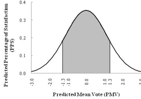
FIG. 2 (b) normalized distribution of PPS versus PMV for 80% satisfaction fall within the range of  $-1.3 < PMV < +1.3$ .
