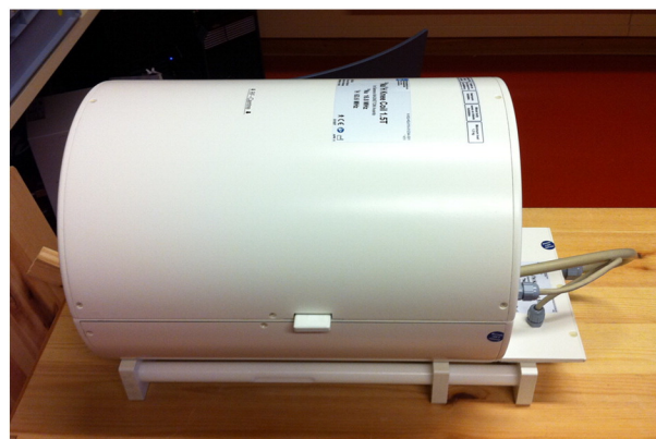
Fig. 3. Dual-tuned knee coil ( ^{23}\text{Na}/^1\text{H} ) equipped with proton channel ( ^1\text{H} -tuned at 63.6 MHz) and sodium channel ( ^{23}\text{Na} -tuned at 16.8 MHz).
