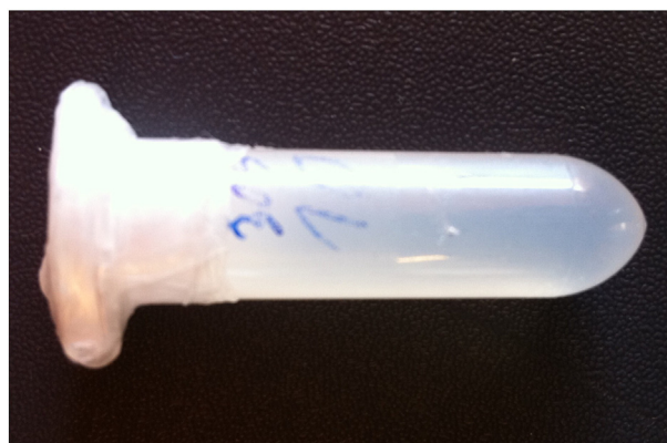
Fig. 4. Calibration reference with sodium concentration of 300 mmol/l.
