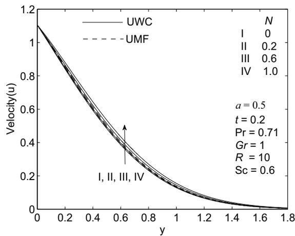
**FIGURE 3.** Velocity Profiles at Various  $N$  (Exponentially Accelerated Plate)
