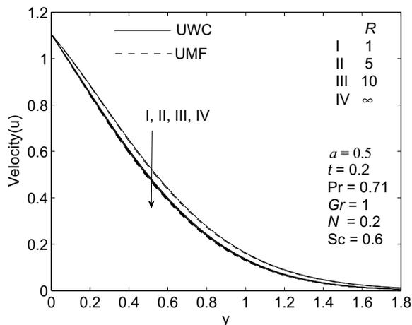
**FIGURE 4.** Velocity Profiles at Various  $R$  (Exponentially Accelerated Plate)
