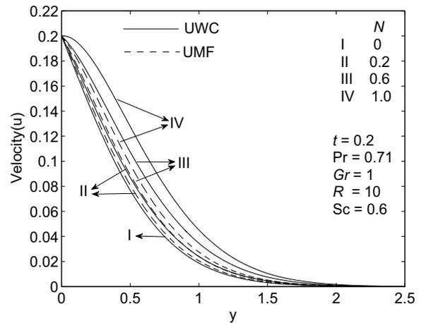
FIGURE 1. Velocity Profiles at Various  $N$  (Uniformly Accelerated Plate)
