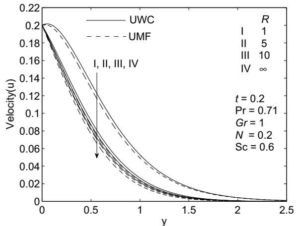
FIGURE 2. Velocity Profiles at Various  $R$  (Uniformly Accelerated Plate)
