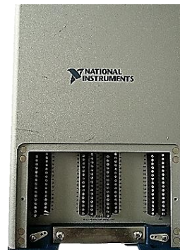
Fig. 2. NI-DAQ –X series signal generation unit for EEG simulation.
