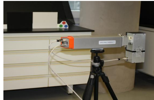
Figure 2. Image acquisition setup with white and black reference plates.
