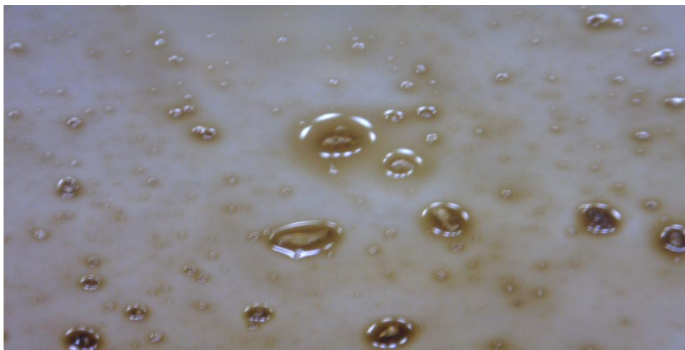
Figure 3. The micrograph of oil-solution precipitated after titration – 200X
