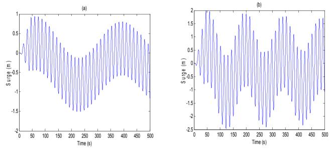
Figure 2. Surge response in regular waves (LC1) a)Classic spar (b)Truss spar
