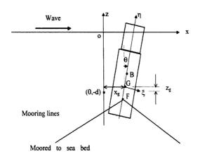
Figure.1 Three-DOF Surge-heave-pitch model of the spar
