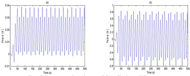
Figure 3. Heave response in regular waves (LC1) (a)Classic spar (b)Truss spar
