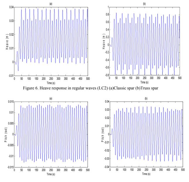
Figure 7. Pitch in regular waves (LC2) (a)Classic spar (b)Truss spar
