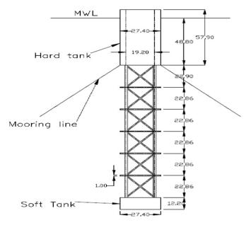
Fig. 4. Overall spar configuration (all dimensions are in m).
