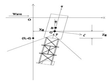
Fig. 3. Global and local coordinates used for dynamic analysis.
