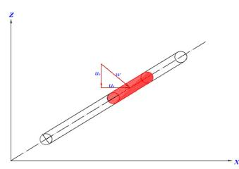
Fig. 2. Wave kinematics components on a segment on inclined cylinder.
