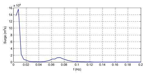
Fig. 6. Surge spectra: mean position (MP)+structure displacement (SD)+drag force (DF).
