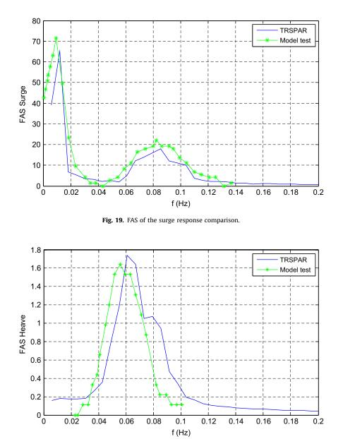
Fig. 20. FAS of the heave response comparison.
