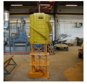
Fig. 17. A typical truss spar model at FORCE Technology.
