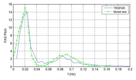
Fig. 21. FAS of the pitch response comparison.
