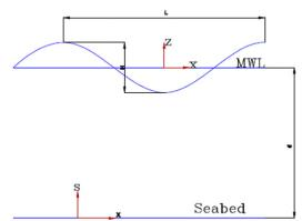
Fig. 1. Definition sketch for a progressive wave train.
