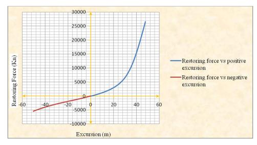
Fig. 5. Quasi-static simulation: restoring force vs. horizontal excursion.
