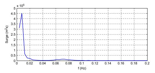
Fig. 10. Surge spectra: MP+SD+DF+AD+FS+CA+temporal acceleration (TA).
