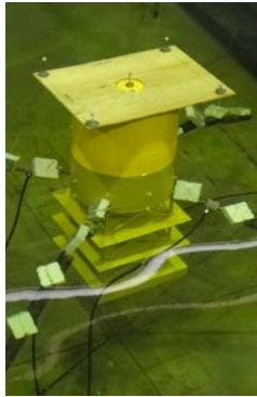
Figure 2 Truss Spar model
