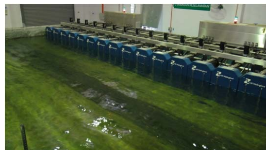
Figure 1 Wave tank facilities - Wave generator
