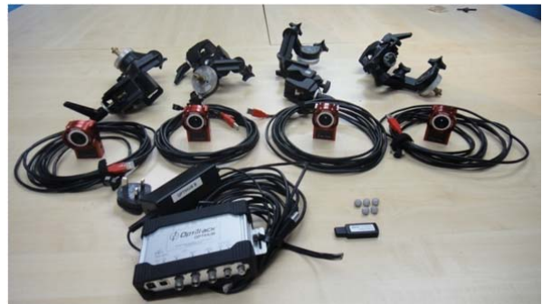
Figure 4 Optical tracking system components
