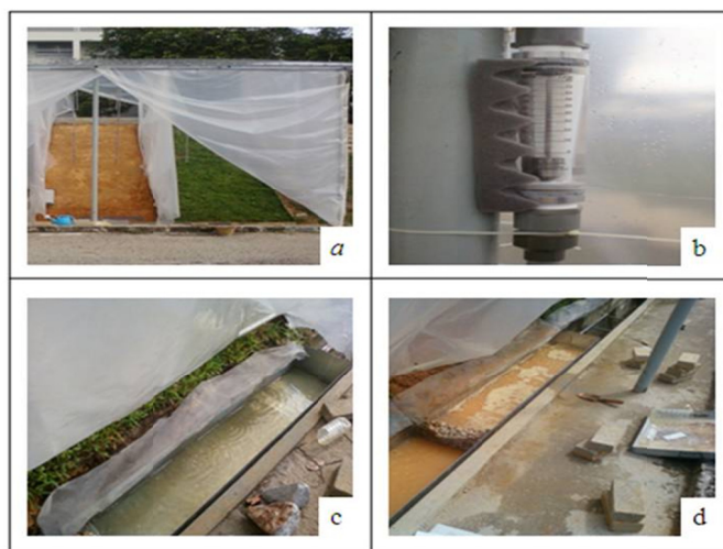
Figure 2. Description of the study area (a) site location of plot-I and plot-II, (b) flow meter, (c) and (d) water samples collected from Plot-I and Plot-II for assessing turbidity and suspended solids
