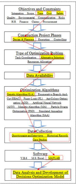
Fig(4): <u>Flow chart for using optimization</u> <u>algorithms for developing decision making</u> <u>framework in construction management.</u>
