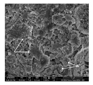
Fig. 7 SEM image of control geopolymer sample: *A* indicates unreacted fly ash particles, and *B* shows amorphous gel phase
