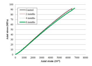
Fig. 6 Stress-strain variation of geopolymer in CO<sub>2</sub>
