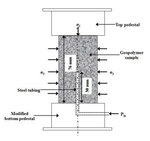
Fig. 4 Schematic diagram of the sample mounted on the *bottom* pedestal
