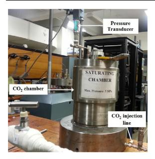
Fig. 1 The CO<sub>2</sub> chamber used to saturate geopolymers
