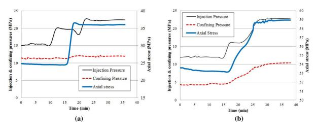
Fig. 10 Variation of applied stresses with injection time for: a Test 1 and b Test 4
