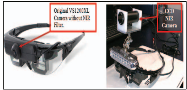
Fig.3. Original Vuzix STAR 1200XL visible light camera (left) and TVL 420 NIR-based CCD camera (right).
