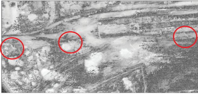
Figure 9. Disparity map using existing Graph-Cut algorithm to detect power pole and vegetation. this image has a lot of noise and some streaking effect. Red circles show that the power poles in white-colour.
