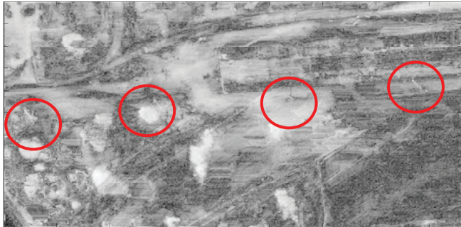
Figure 10. Disparity map using proposed Graph-Cut algorithm incorporated with ordering constraint has less noise and detect power poles to some extent. Red circles show that the power poles in white-colour.
