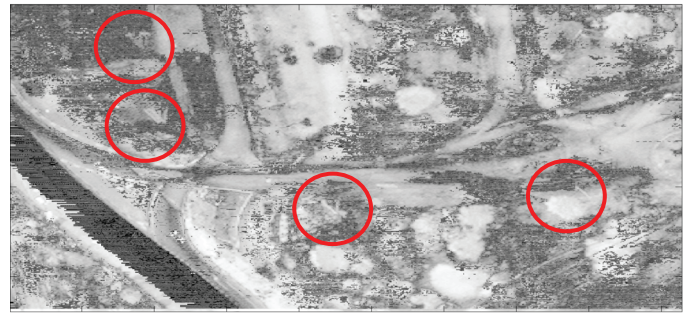
Figure 5. The disparity map obtained using existing Graph-Cut Algorithm on Pleiades satellite stereo image has some noise in textureless areas and not smooth. Red circles show that the power poles in white-colour.
