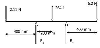
Figure 11. Free body diagram of the forces acting at  $R_3$  and  $R_4$
