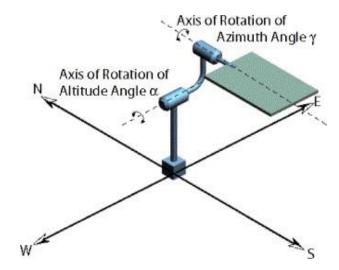
Figure 1. Two axis azimuth/elevation sun tracking system
