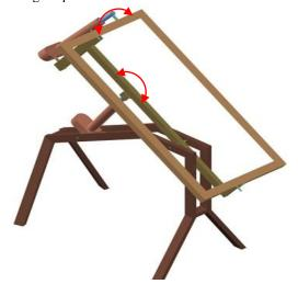
Figure 14. Illustration of azimuth and elevation tracking directions
