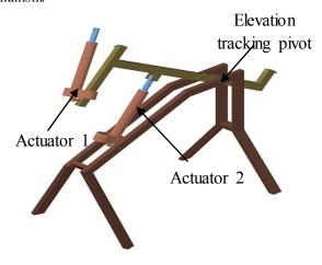
Figure 10. Actuators and the hinge mechanism
