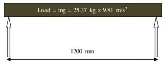
Figure 6. Load analyses of the panel seat and solar panels as Distributed load
