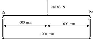
Figure 7. Concentrated load analyses of the panel seat and solar panels
