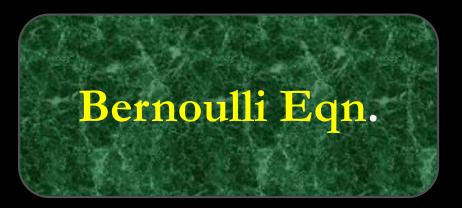
$$\frac{p_1}{\rho g} + \frac{v_1^2}{2g} + z_1 = \frac{p_2}{\rho g} + \frac{v_2^2}{2g} + z_2 + h_l$$
