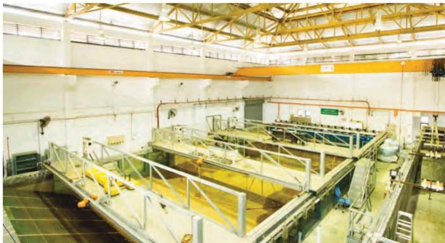
The deep water wave tank in the offshore engineering lab at UTP.
