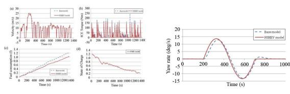
**Fig. 11.** Combined simulation results (a) Velocity profile comparison (b) ICE torque comparison (c) Fuel use comparison (d) SoC of HEV model
