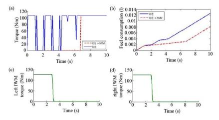
**Fig. 13.** Fuel consumption during cornering results (a) ICE torque comparison (b) Fuel use comparion (c) Left IWM torque (d) Right IWM torque
