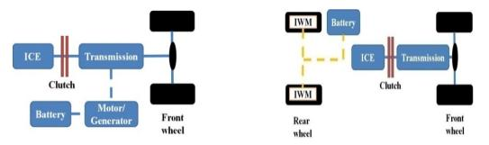
Fig. 1. Common parallel hybrid used by other researchers
