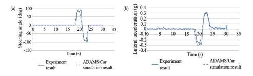
Fig. 8. Results for single lane change test (a) Steering wheel input (b) Lateral acceleration
