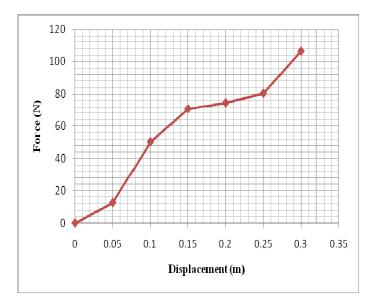
Fig. 3 Force-displacement relationship of the mooring lines
