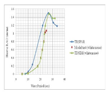
Fig. 9 Comparison of heave RAO at zero degree heading
