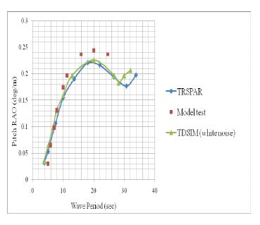
Fig. 10 Comparison of pitch RAO at zero degree heading
