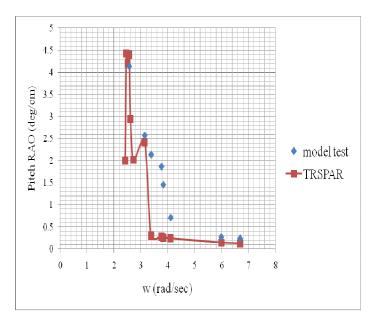
Fig. 7 Comparison of pitch motion RAO
