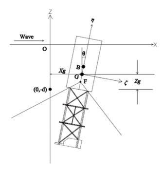
Fig. 4 Three-DOF surge-heave-pitch model of the spar
