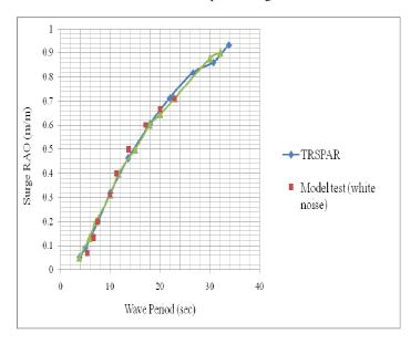
Fig. 8 Comparison of surge RAO at zero degree heading
