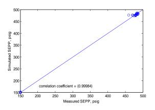
Figure 3. Crossplot of Simulated vs. Measured SEPP (ANN model)
