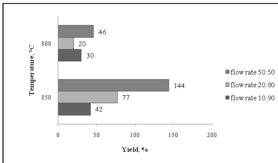
**FIGURE 4.** A comparison of yield gain at different flow rate versus temperature with 0.1 g ferrocene
