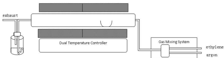
**FIGURE 1.** Schematic diagram of the FCCVD system
