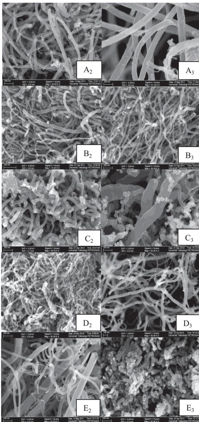
FIGURE 7. SEM images of each sample at 50K magnification except B<sub>2</sub> at 70K
